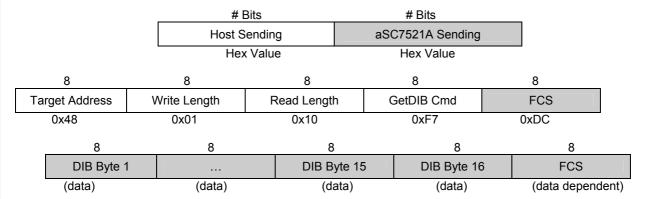
Figure 3. GetDIB() Command (16-byte read length)
