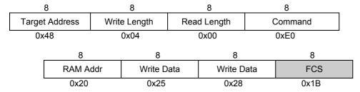
Figure 9. Example Register Write
