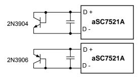
**Figure 17 Discrete Remote Diode Connection**
