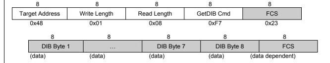
Figure 4. GetDIB() Command (8-byte read length)
